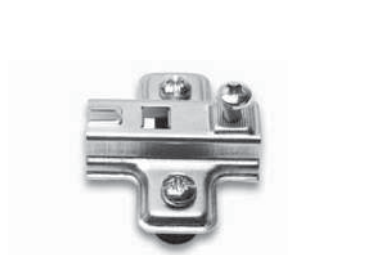
Metal cruciform mounting plate. Knock-in fixing with dowels Ø10mm. Vertical adjustment.
