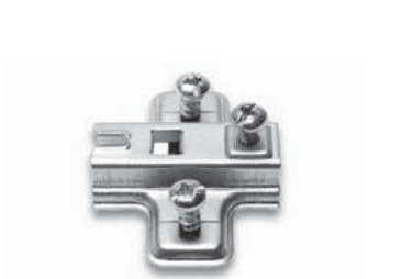
Metal cruciform mounting plate. Fixing by expanding X-Pando dowels Ø5mm. Vertical adjustment.
