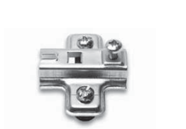
Metal cruciform mounting plate. Knock-in fixing with dowels Ø8mm. Vertical adjustment.
